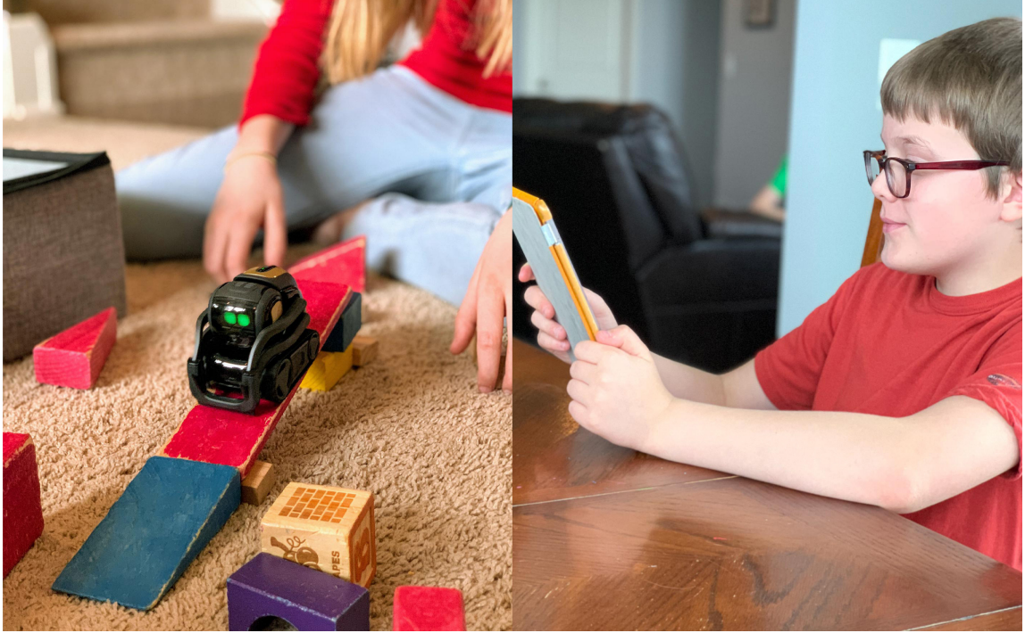
Figure 4.1: Remote Social Play with VectorConnect. A child (right) engages in remote physical play using our system, which enables real-time control of and communication through a Vector robot located in their peer’s environment (left). The system facilitates physically playful and socially interactive experiences across geographic distance.
