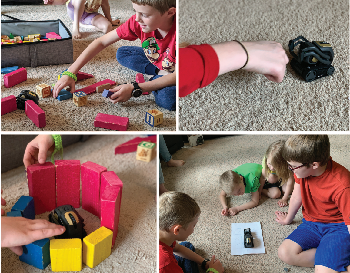
Figure 4.3: System Usability Testing with Children. In this pilot session, children explored the system’s ease of use through suggested and self-directed play scenarios. As shown from left to right, they built obstacle courses using household objects, greeted remote peers via robot fistbumps, played hide-and-seek by hiding the robot, and engaged in a game of tic-tac-toe through remote teleoperation.
